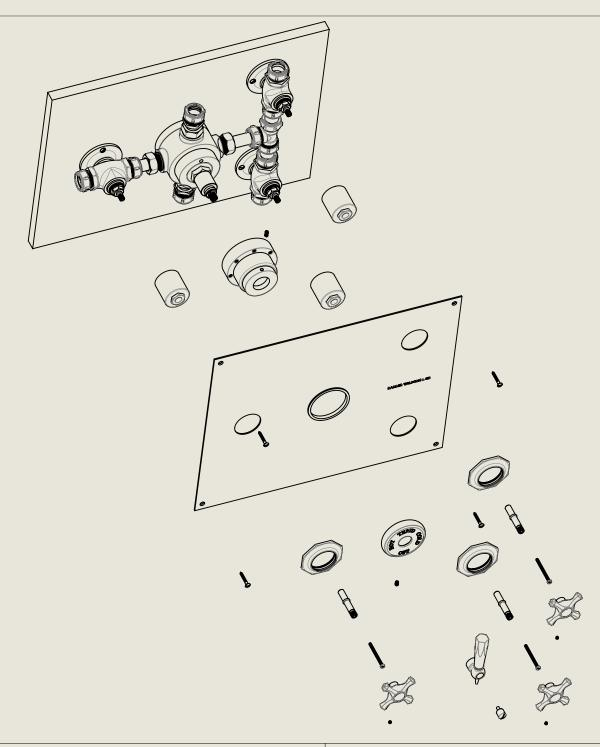
An additional extension is available to extend tolerance to 20mm
